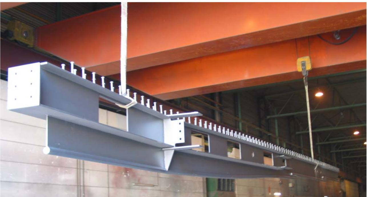
Figure 18. DEXIA-BIL building A; specially shaped composite floor beam at fabrication shop of Victor Buyck, Eeklo (B), in November 2004
