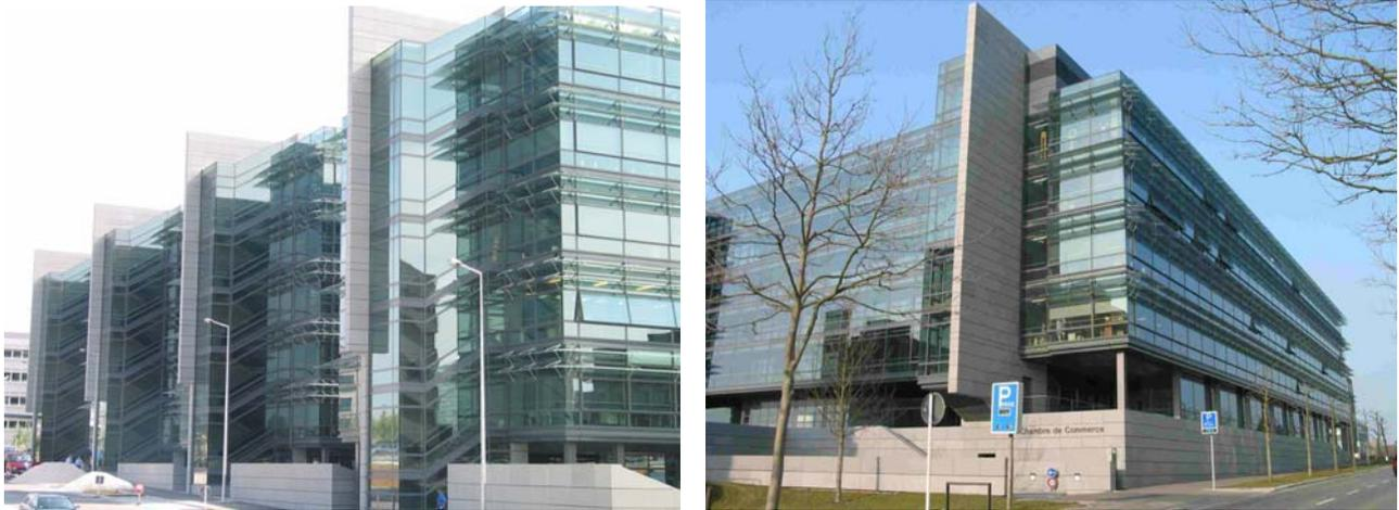
Figures 4 and 5. Glass façades with solar radiation deflectors
