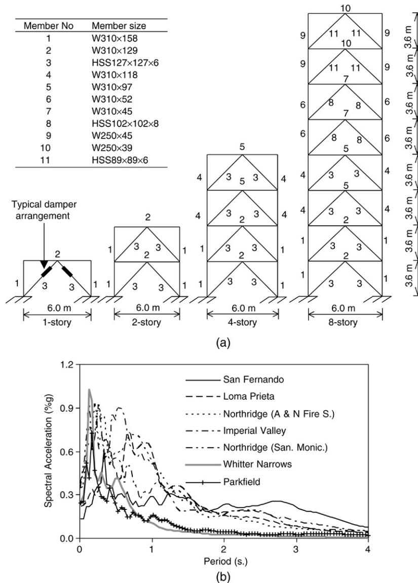
Fig. 1. (a) Frame models. (b) Acceleration response spectra of the earthquakes used in the analyses.
