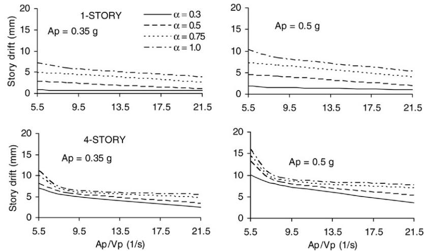
Fig. 9. Maximum inter-story drifts of one and four-story CBFs with VFDs as a function of the  $A_p/V_p$  ratio of the ground motion for various  $\alpha$  values and  $A_p = 0.35$  and  $0.50$ g.
