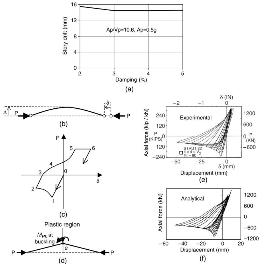
Fig. 3. (a) Story drift of one-story frame versus structural damping ratio. (b) Buckling brace. (c) Typical brace axial force–deformation behavior. (d) Nonlinear brace model. (e) Experimental hysteresis loop. (f) Analytical hysteresis loop from ADINA [21].
