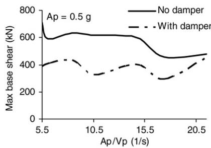
Fig. 6. Comparison of the maximum base shear forces vs.  $A_p/V_p$  ratio of the ground motion for a one-story frame.
