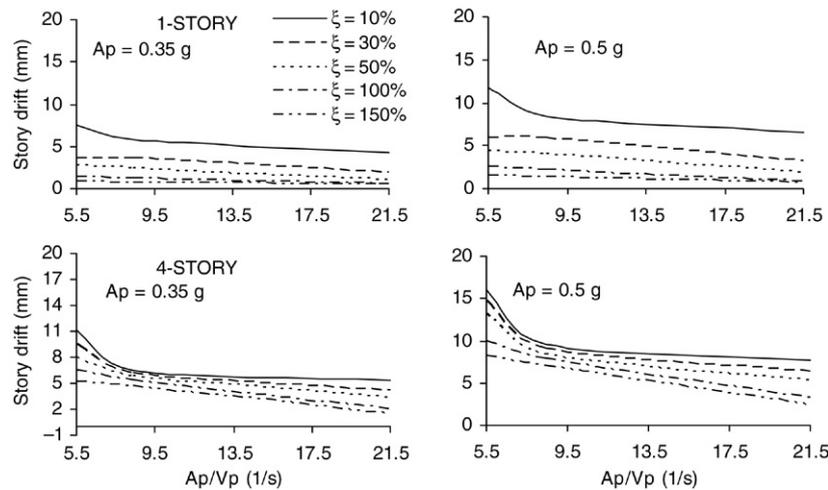
Fig. 7. Maximum inter-story drifts of one and four-story CBFs with VFDs as a function of the  $A_p/V_p$  ratio of the ground motion for various damping ratios and  $A_p = 0.35$  and  $0.50g$ .
