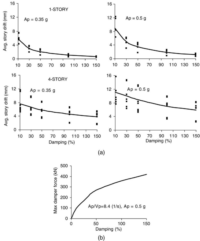
Fig. 8. (a) Average of the maximum inter-story drifts of CBFs with VFDs from the seven earthquakes as a function of the damping ratio for one and four-story frames and  $A_p = 0.35$  and  $0.50$ g. (b) Maximum damper force as a function of the damping ratio for one-story frame.
