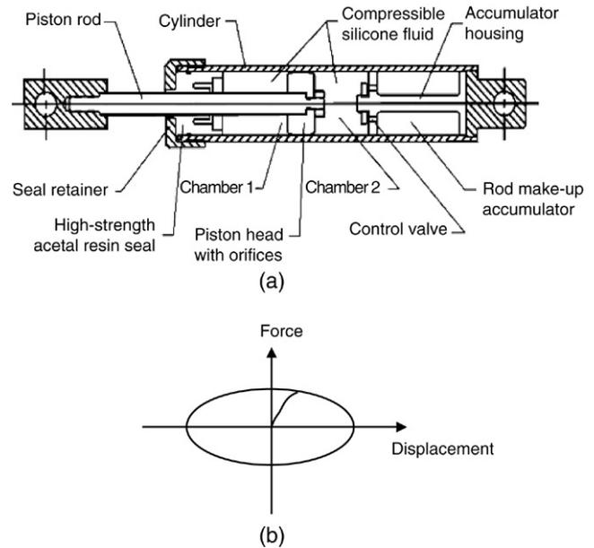
Fig. 2. (a) Typical detail of a viscous fluid damper. (b) Force–displacement loop of a viscous fluid damper.
