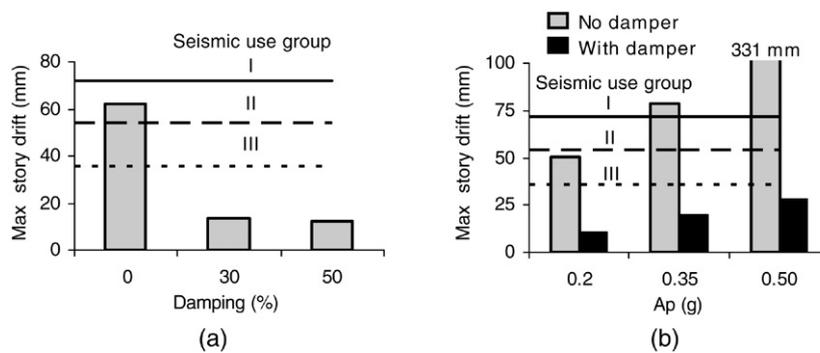
Fig. 11. (a) Comparison of code mandated allowable drifts with those of a four-story CBF without VFDs and with VFDs having various damping levels ( $A_p = 0.50g$ ,  $A_p/V_p = 6.1 s^{-1}$ ). (b) Comparison of code mandated allowable drifts with those of an eight-story CBF with and without VFDs for various  $A_p$  values ( $A_p/V_p = 5.5 s^{-1}$ ).
