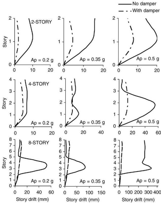
Fig. 5. Displacement profile of the two, four and eight-story CBFs with and without VFDs for various  $A_p$  ( $A_p/V_p = 5.5 \text{ s}^{-1}$ ).
