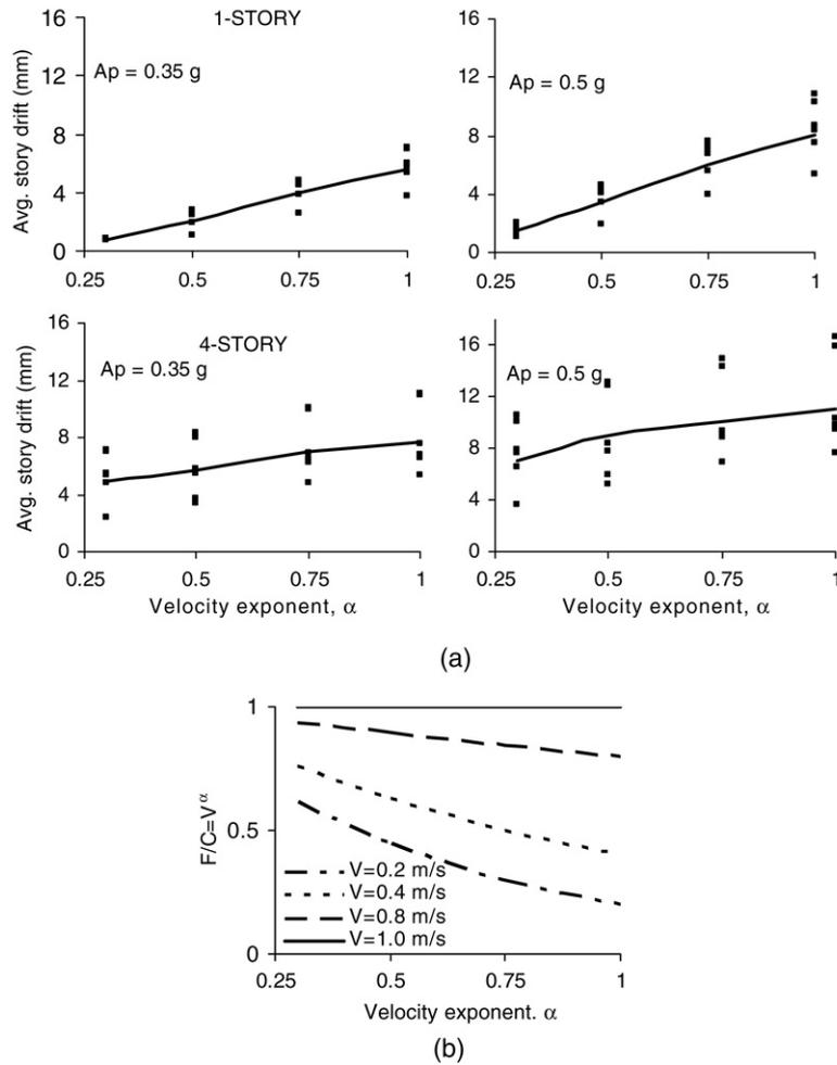
Fig. 10. (a) Average of the maximum inter-story drifts of CBFs with VFDs from the seven earthquakes as a function of the damper velocity exponent for one and four-story frames and  $A_p = 0.35$  and  $0.50g$ . (b) Variation of normalized damper force with respect to  $C$  as a function of velocity exponent for various damper velocities.
