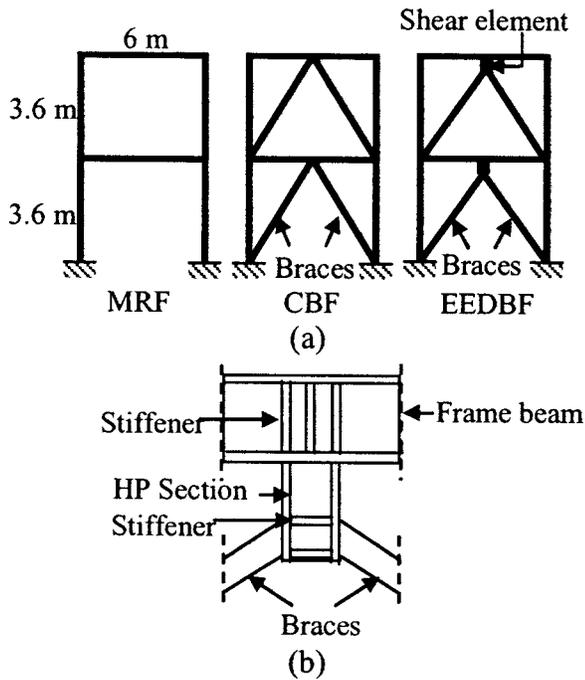
**Fig. 1.** (a) Typical two-story frames; (b) details of shear element and connections in EEDBF
