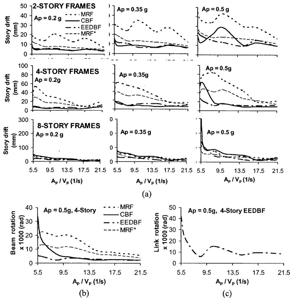
**Fig. 9.** (a) Maximum interstory drift versus  $A_p/V_p$  ratio of the ground motions for various  $A_p$  for the two-, four- and eight-story frames; (b) beam-end rotations versus  $A_p/V_p$  for the four-story frames; and (c) link rotation versus  $A_p/V_p$  for the four-story EEDBF
