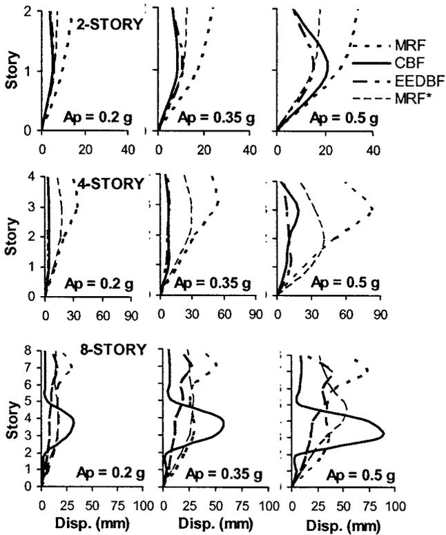
Fig. 10. Displacement profile of the two-, four-, and eight-story frames for various  $A_p$  ( $A_p/V_p=8.4 \text{ s}^{-1}$ )
