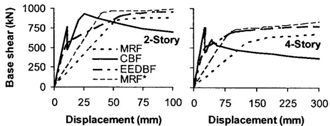
**Fig. 8.** Base shear versus top displacement for two- and four-story frames
