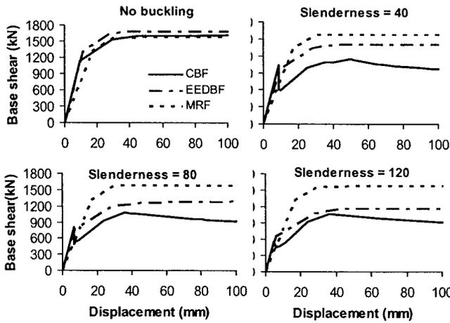
Fig. 4. Base shear versus frame displacement for various brace slenderness ratios
