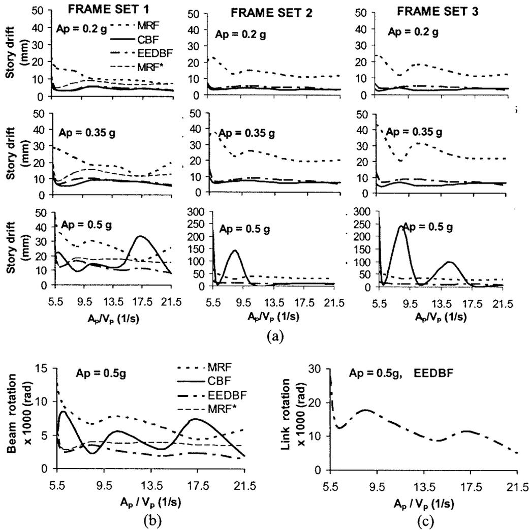
**Fig. 6.** (a) Maximum story drift versus  $A_p/V_p$  ratio of the ground motions for the three frame sets and for various  $A_p$ ; (b) beam-end rotations versus  $A_p/V_p$  for Frame Set 1; and (c) link rotation versus  $A_p/V_p$  for the EEDBF in Frame Set 1
