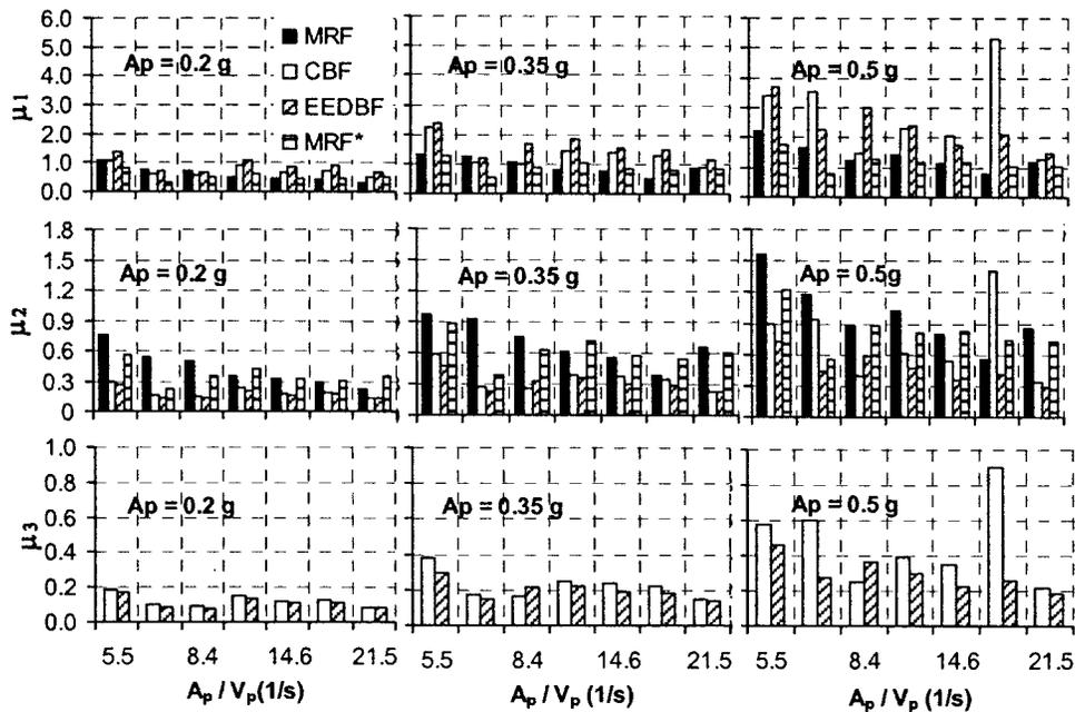
Fig. 7. Ductility ratios as a function of  $A_p/V_p$  ratio of the ground motions for various  $A_p$
