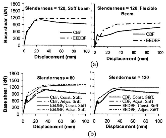
Fig. 5. (a) Effect of beam stiffness on force-displacement response and (b) effect of brace stiffness on the force-displacement response
