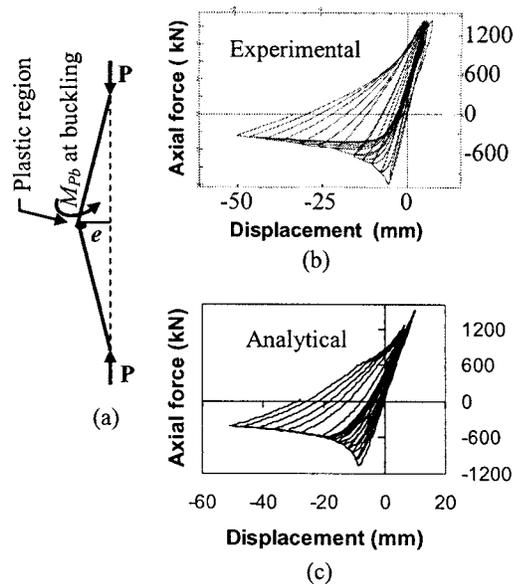
**Fig. 3.** (a) Nonlinear brace model; (b) experimental hysteresis loop (Black et al. 1980, reprinted with permission); and (c) analytical hysteresis loop generated by using ADINA (2004)
