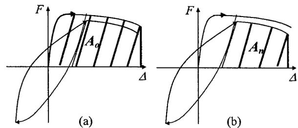
Fig. 12. Definition of damage equation parameters of the model by Hindi and Sexsmith (2001): (a) monotonic energy in the virgin state; (b) monotonic energy after the application of load-displacement cycles
