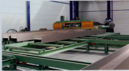
2. Peddinghaus DG 1100 gönyeyburun testeresi
