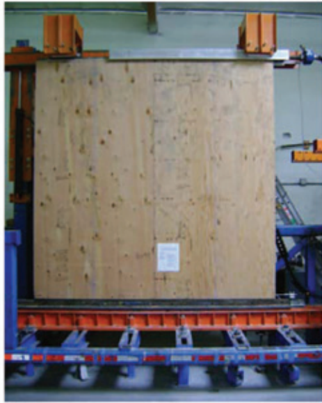
Figure 5. Shear wall test set-up
