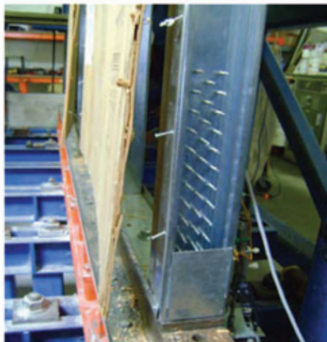
Figure 6. Plywood pull-over failure for full-scale CUREE tests
